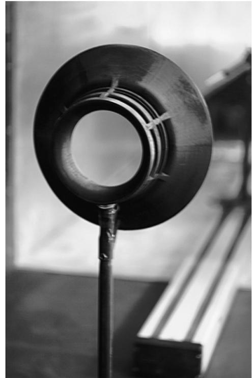
Fig. 11. The  $\nu 11$  1:20 scale experimental model placed in the TASL 2 experimental vein. The traversing system and the static pressure probe are shown in the far plane.
